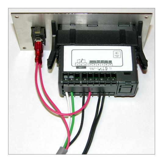
Thermostat Electrical Wiring Connections (Shown assembled with the On/Off rocker switch in the mounting bracket) 2. The temperature probe (015-0002, black wires on right side) attaches to the Carel thermostat connections 7 and 8.
