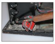
11. De-burr the end of the condenser discharge tube. Carefully bend the condenser discharge tube back to near where it was before removing the old filter-drier.
