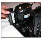
plastic housing of the module over the flange on the condenser side of the module mounting bracket. The module will fit around this flange, and the screw hole on the power module will align with the screw hole on the compressor module mounting bracket. Attach the module housing over the bracket, insert the screw through the hole in the module housing and into the threaded hole in the bracket on the compressor, and tighten the screw with a screwdriver.
