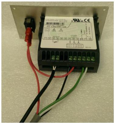
Thermostat Electrical Wiring Connections (Shown assembled with the On/Off rocker switch in the mounting bracket)
