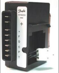
3. Fan: There should also be fan or water pump wiring on the module terminal connections "F" and small "+". This circuit has a continuous current capacity of 1/2 amp and a peak capacity of 1 amp.
